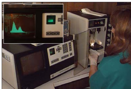
Blood samples are analyzed using a Coulter Counter Particle Sizer with Channelizer.
