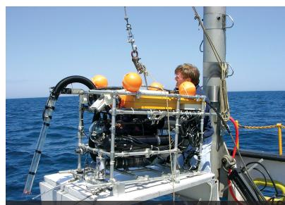
Using a remotely operated vehicle sampler, scientists are able to quantify the density of fall and spring sac fry to determine success of natural reproduction. Photo courtesy of J. Janssen.
